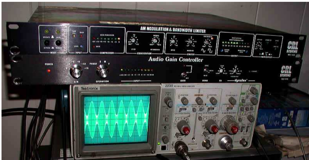
Sinewave 75% modulation through entire system, audio processing on top of scope.
