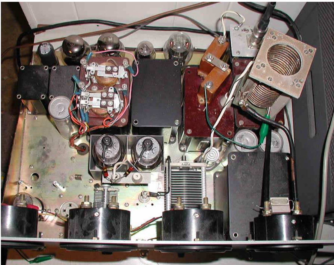
Side view of the transmitter with new Output network at far end.
