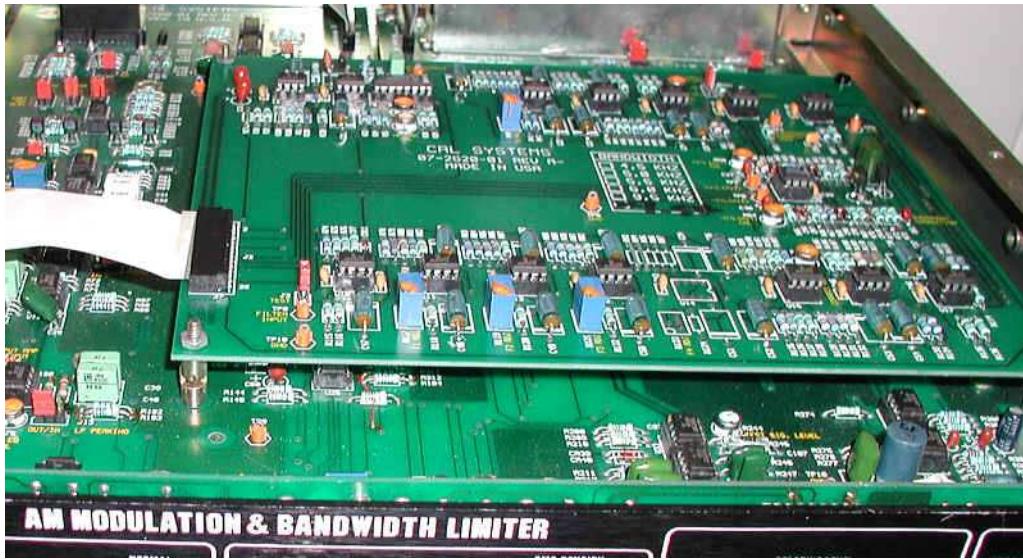
Special 3.2 kHz audio output filter board in MBL audio processor unit.
