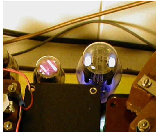
0D3 / VR150 voltage regulator and Type 83 Mercury Vapor HV rectifier.
